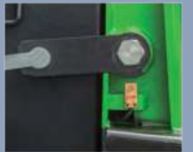
The tow tractor has a safety feature where it can only travel if the battery locking pin is correctly rotated.
