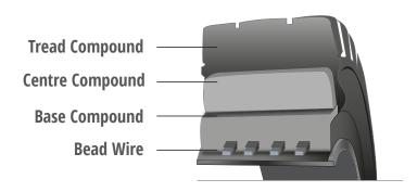
With better handling, stable cornering and a highly functional design, GLOBESTAR WT is ideal for electric and internal combustion engine forklifts operating in regular material handling applications. GLOBESTAR WT tires are also reinforced with creel bead wires to ensure secure wheel and rim fitment.
