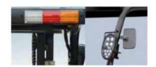
The new efficient lighting system uses LEDs and a new type of reflector to reduce energy consumption. This significantly improves illumination performance while also prolonging operation time.
