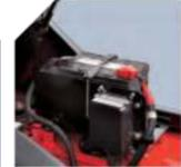
The controllers, relays, and safety fuses are all placed in the dust and water-free controller box. The main electronic components are also all waterproof. This allows the operator to use the forklift in wet environments.
