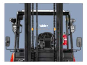
The mast was redesigned to provide broad forward visibility. This was done by increasing the distance between the inside of the mast by 2.34".
