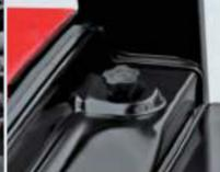
The location of the air filter allows for easy reach and replacement when the filter needs to be changed.
