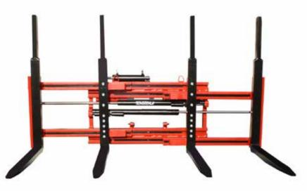
Multiple Pallet Handler are used in all industries characterized by heavy handling of palletized loads and in particular warehouse, food and beverage, and brick industries.
